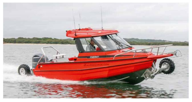
The Stabicraft 2100 ST comes in a hardtop version for all-weather protection and a comfortable cuddy cabin with three-quarter cushioned bunks. The helm and passenger seats have flip-up bolsters for standing comfort and there's a full array of instrumentation on the dash, including the Sealegs control. A Simrad evo2 GPS chartplotter/sounder, stereo sound system and Simrad VHF radio complete the fitout.
