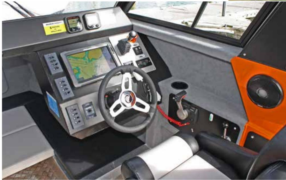
Above: The large 12in Lowrance display is prominent at the helm, as are the driving controls for the Sealegs amphibious system.
