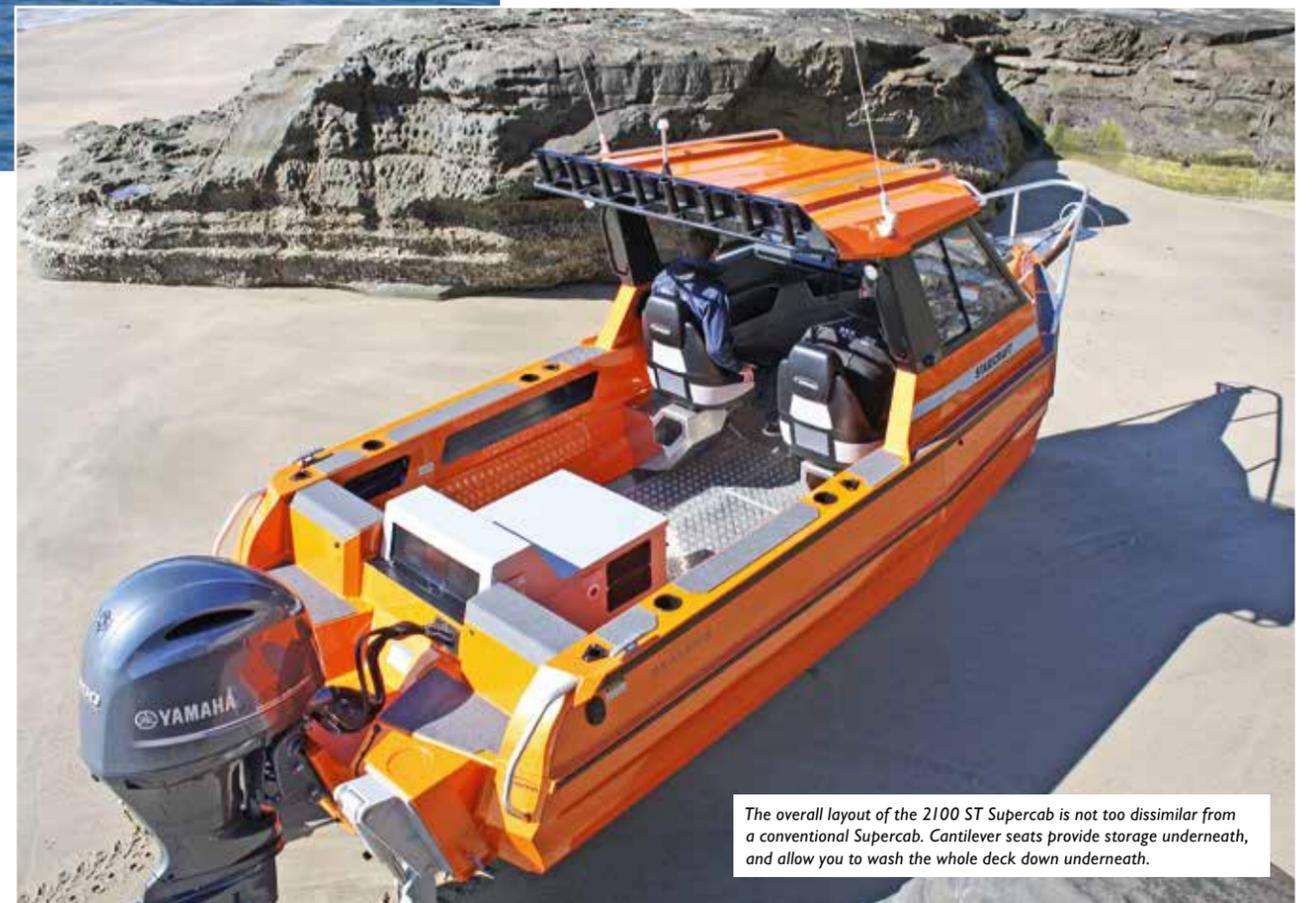
The overall layout of the 2100 ST Supercab is not too dissimilar from a conventional Supercab. Cantilever seats provide storage underneath, and allow you to wash the whole deck down underneath.
