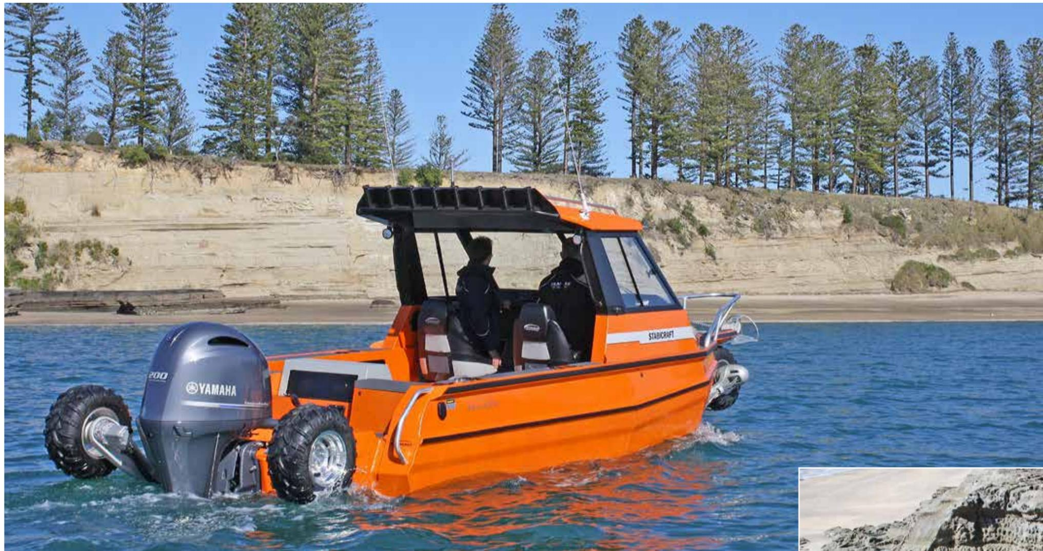
Above: The Yamaha F200 four-stroke outboard will push the 2100 ST along to 37 knots.
