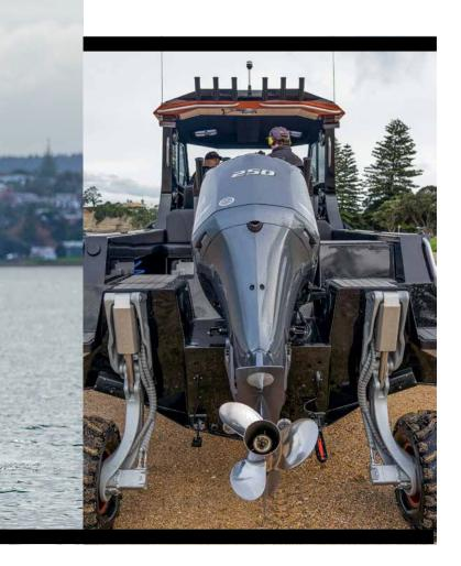
accessible via a hatch on the starboard side. The step-through is on the port side where the transom is slightly lower. The boarding ladder is designed not only for boarding the boat from the water, but also from land. Folding to the side, the ladder is shaped to clear the rear wheel.
