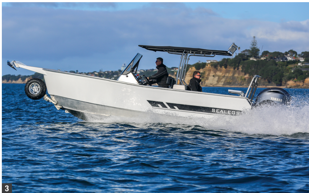
1) The targa top can be folded down to rest on the ski rail above the outboard, making garaging a simple proposition. 2) The 7.5m Alloy Centre Console is based on the well-proven hull of the Sealegs 7.5m Amphibious RIB. 3) The Yamaha 225hp provided plenty of boogie, topping out at over 40 knots.
